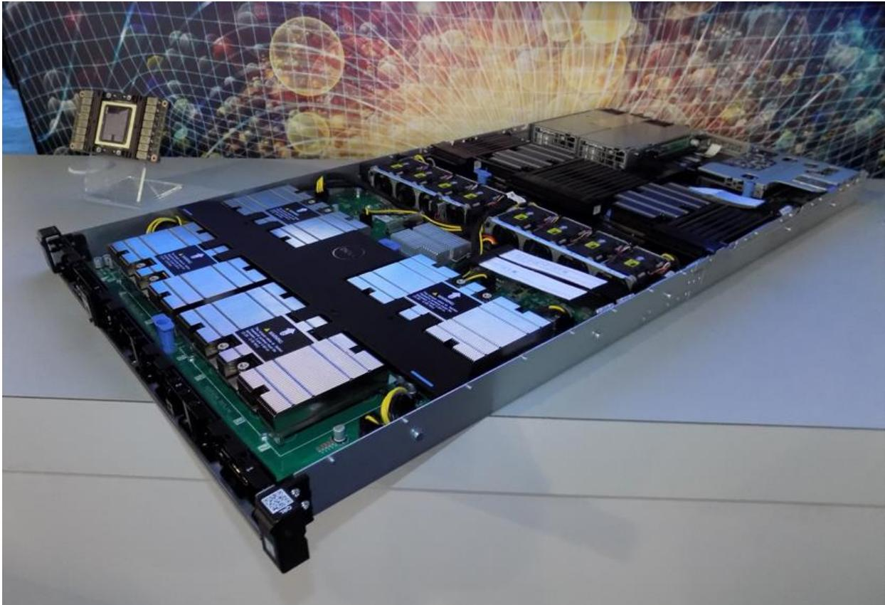
*The Dell EMC PowerEdge C4140 is designed specifically to support the compute needs of HPC and Machine Learning with two Intel Scalable Xeon CPUs and four NVIDIA GPUs interconnected over NVLINK.*
