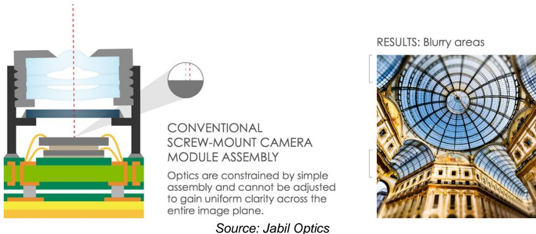
Active alignment is a dynamic method of affixing an optical array in an optical image assembly. This method usually incorporates image data from the sensor through a feed that allows the machine to adjust for imperfections and optimize the alignment across the entire image plane. Depending on the manufacturing needs of the customer and the capabilities of the equipment and software, active alignment results in higher precision manufacturing and image quality.
