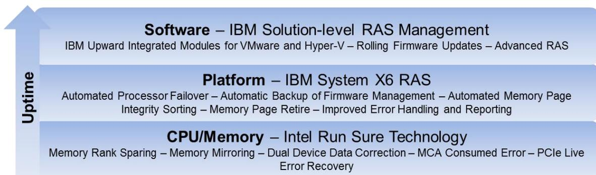
The Run Sure Technology features bring the Machine Check Architecture that RISC and Itanium systems have had for years into an x86 platform. These features help the
