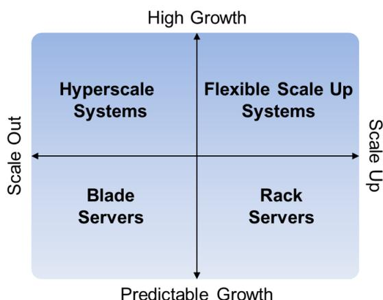
In stable growth environments, traditional rack and blade servers are fine depending on whether applications will need to scale up with rack systems (larger memory footprints, more/faster CPUs, or more internal storage) or scale out with blades (more dense physical systems to spread the workload).
