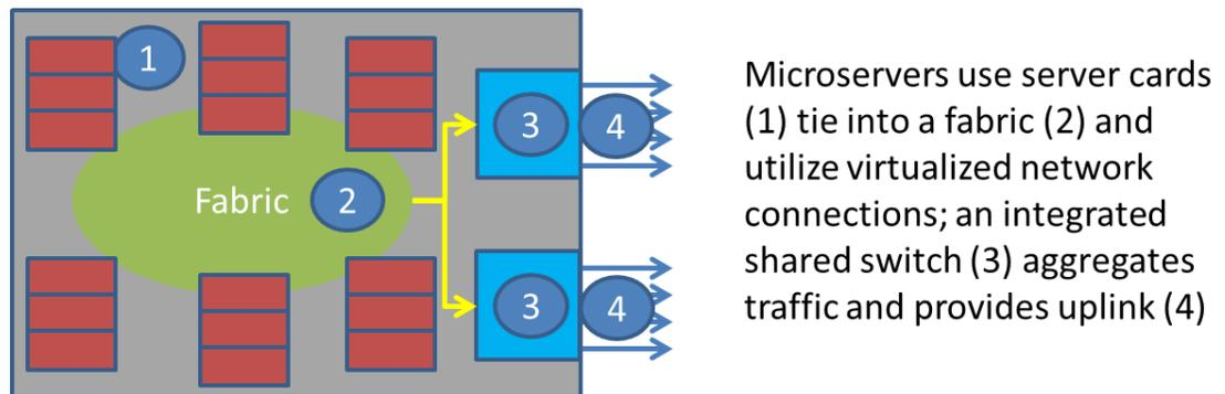
Microservers use server cards (1) tie into a fabric (2) and utilize virtualized network connections; an integrated shared switch (3) aggregates traffic and provides uplink (4)
