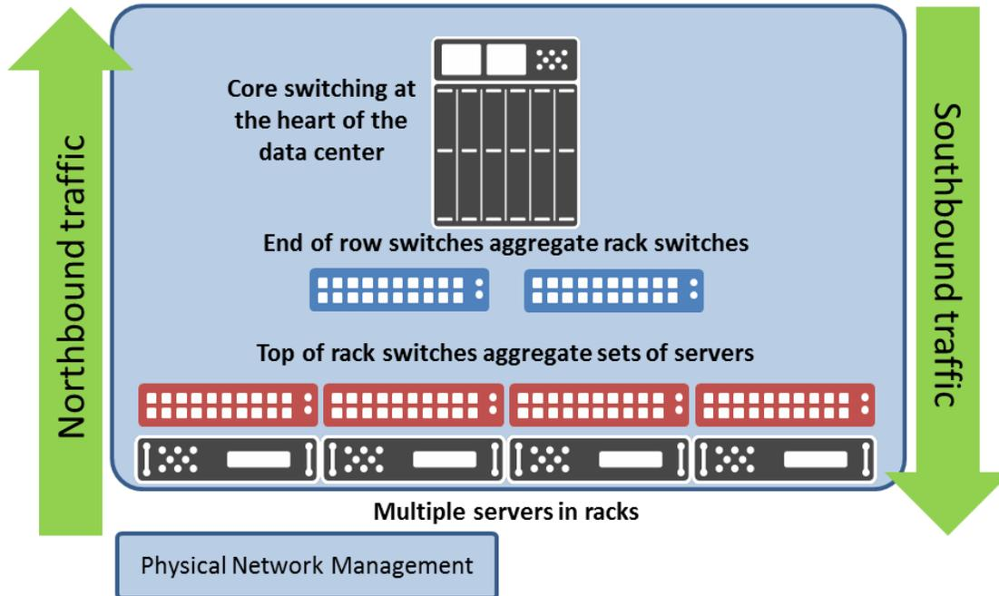
In an SDN environment, the SDN management tool manages the virtual layer and the standard management tool manages the underlying physical layer:
